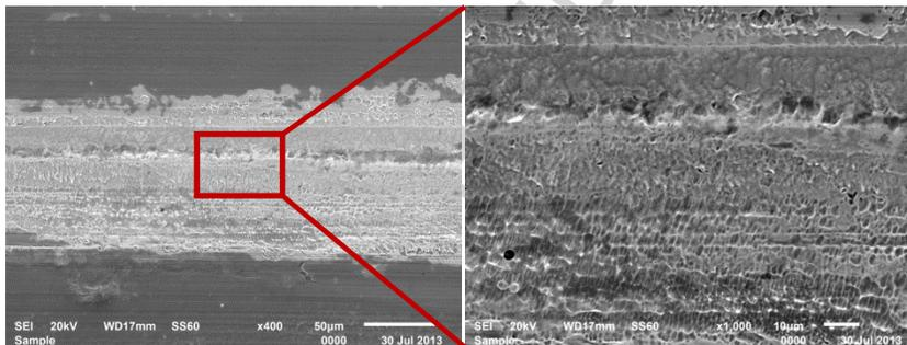
Figure 4: SEM micrographs of case #3 at 400x and 1000x magnification showing corrosion pits.
