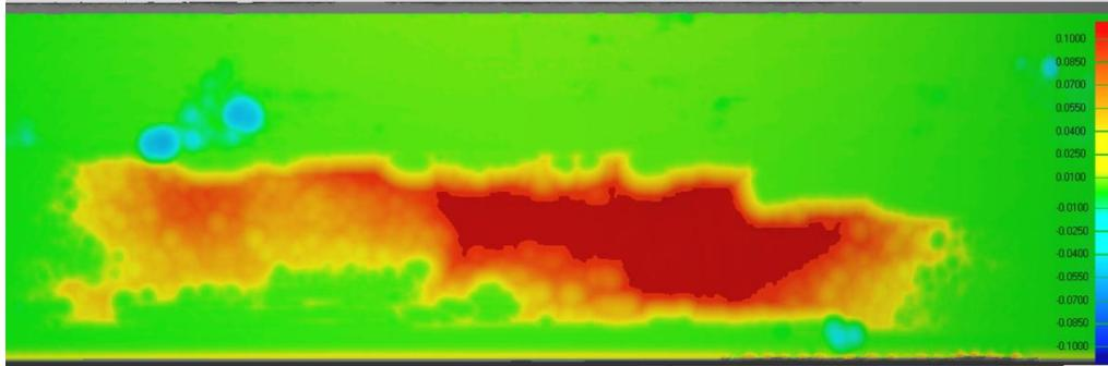
Figure 2: Colour deviation map of the corrosion scar of case #8.
