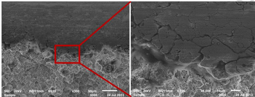
Figure 3: SEM micrographs of case #8 at 300x and 1000x magnification demonstrating crevice corrosion at the grain boundaries.
