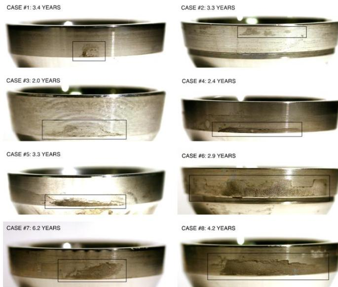
Figure 1: Photographs of the 8 cases of liner corrosion with implantation period.
